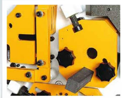
Bar Shearing Station
